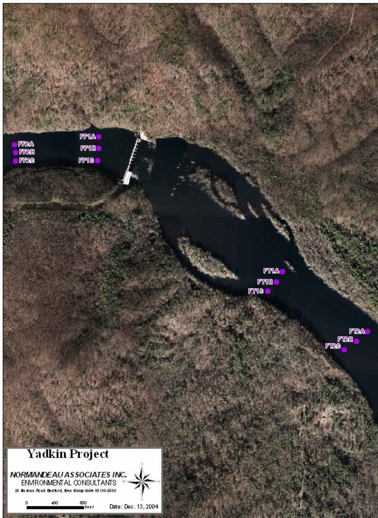
Figure 3.4-4. Location of transects/sampling stations for lateral and longitudinal survey of dissolved oxygen and temperature at Falls.
