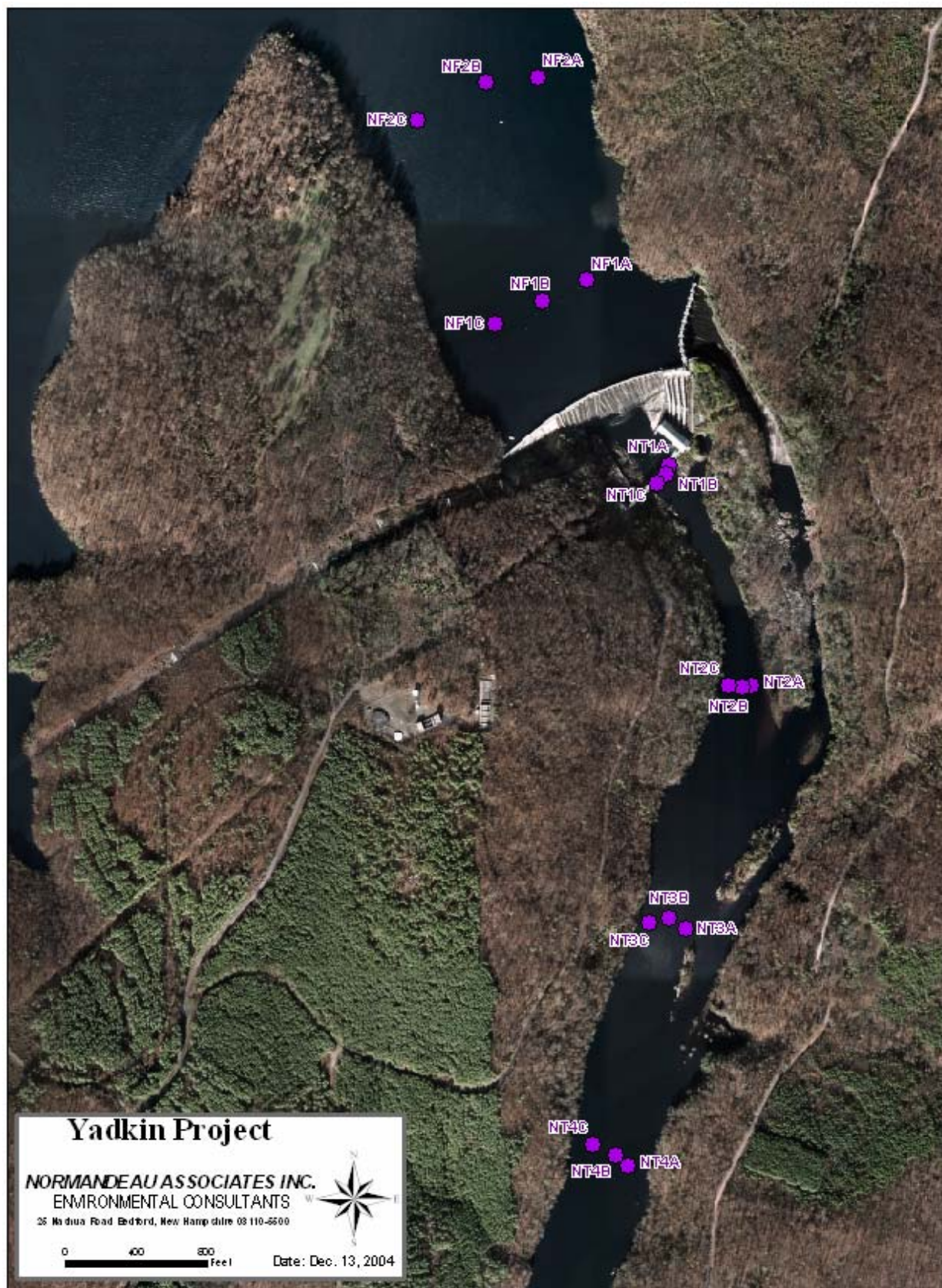
Figure 3.4-3. Location of transects/sampling stations for lateral and longitudinal survey of dissolved oxygen and temperature at Narrows.
